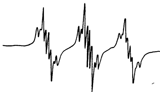
Fig. 1. ESR spectrum of m -BuNOPSt in toluene solution (1%) taken at 80°C.
